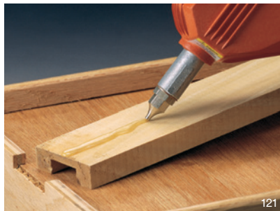
For bonding the guide to a drawer bottom, 3M™ Hot Melt Adhesive 3792 provides high delivery rate and long bonding range.
