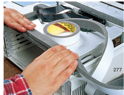
When compressed 50%, the open cell construction of 3M™ Urethane Foam Tape 4314 provides an air barrier and cushion in electronic equipment.
