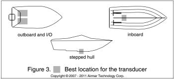
starboard side of the hull where the propeller blades are moving downward is preferred.
