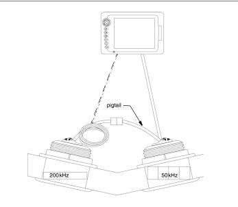
Figure 4. Connecting a Pair—single transmission line Copyright © 2008 Airmar Technology Corp.
