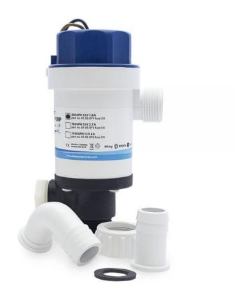
Twinport cartridge aerator pump 12V with flowrate 50l/min (750GPH). The twinport makes it possible to use the same intake 19mm (3/4") for both the livewell and wash down pump. Equipped with both straight and elbow 19mm (3/4") detachable ports. Amperage 2,7A, fuse size 5A.
