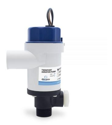
Twinport cartridge aerator pump 12V with flowrate 75l/min (1100GPH). The twinport makes it possible to use the same intake for both the livewell and wash down pump. Equipped with straight fixed 29mm (1,15") port. Amperage 4A, fuse size 5A.
