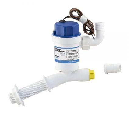
Cartridge Aerator Pump 12V with flowrate 32l/min (500GPH) with angeled intake. Equipped with both straight and elbow 19mm (3/4") detachable ports. Amperage 1,8A, fuse size 5A. Easy to install, maintain and to replace the cartridge.
