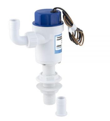
Cartridge Aerator Pump 12V with flowrate 50l/min (750GPH) with straight intake. Equipped with both straight and elbow 19mm (3/4") detachable ports. Amperage 2,7A, fuse size 5A. Easy to install, maintain and to replace the cartridge.
