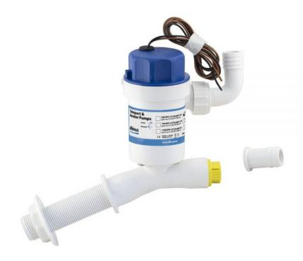
Cartridge Aerator Pump 12V with flowrate 50l/min (750GPH) with angeled intake. Equipped with both straight and elbow 19mm (3/4") detachable ports. Amperage 2,7A, fuse size 5A. Easy to install, maintain and to replace the cartridge.
