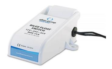
The 12/24/30V bilge float switch activates your bilgepump automatically when water exceeds the acceptable level and deactivate when water has been removed. For a fully automatic removal of your bilge water connect a switch to your electrical bilge pump. Safe removal of bilgewater when nobody is onboard, approved for 500 000 cycles. 14A.
