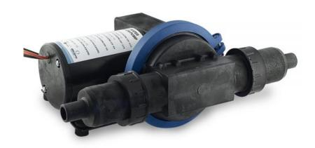
Single chamber, self priming, diaphragm pump 12V for grey or bilge water. Shower drain, transfer or pump out. Capacity 22 L/min (5,8 GPM), flexible installation with 360 degree rotational ports. Quiet operation and low power consumption. Operates with no need for filter. Including 19mm (3/4") and 25mm (1") straight connectors. 4,5A fuse. Interchangeable with Johnson Pump 10-13350-03.
