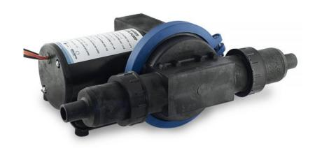
Single chamber, self priming, diaphragm pump 24V for grey or bilge water. Shower drain, transfer or pump out. Capacity 22 L/min (5,8 GPM), flexible installation with 360 degree rotational ports. Quiet operation and low power consumption. Operates with no need for filter. Including 19mm (3/4") and 25mm (1") straight connectors. 2,5A fuse. Interchangeable with Johnson Pump 10-13350-04.
