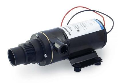
Macerator Pump 12V equipped with rotary cutter and impeller to discharge waste water with high capacity. Capacity 43 L/min (11,5 GMP) output at 4 m total head. Self priming up to 1,5 m vertical lift. Brass and stainless steel internal parts and pump body in thermo polymer with a long lasting impeller. Inlet port 38mm (1,5") and outlet 25mm (1"). Amperage 12A. Interchangeable with Jabsco 18590-2092, Johnson Pump 10-24453-04.
