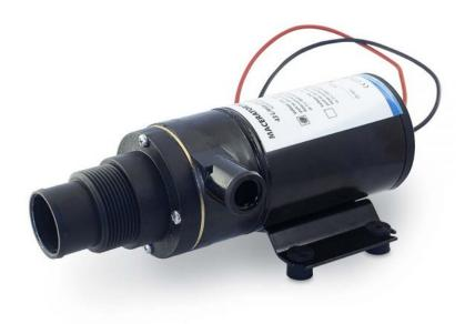
Macerator Pump 24V equipped with rotary cutter and impeller to discharge waste water with high capacity. Capacity 43 L/min (11,5 GMP) output at 4 m total head. Self priming up to 1,5 m vertical lift. Brass and stainless steel internal parts and pump body in thermo polymer with a long lasting impeller. Inlet port 38mm (1,5") and out 25mm (1"). Amperage 7A. Interchangeable with Jabsco 18590-2094, Johnson Pump 10-24453-05.
