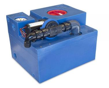
Complete waste water tank kit with pump ready to install. Including a 47L (12,5 G) rectangular tank in reinforced polyethylene, waste water diaphragm pump 12V, gas vent, active carbon filter, control panel and probe for level control. Linear low density polyethylene is the best suited material for holding tanks because of resistance to corrosion and odor permeation.
