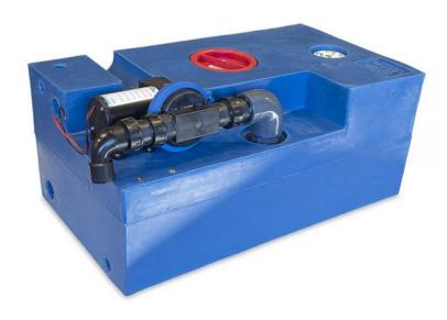
Complete waste water tank kit with pump ready to install. Including a 72L (19 G) rectangular tank in reinforced polyethylene, waste water diaphragm pump 12V, gas vent, active carbon filter, control panel and probe for level control. Linear low density polyethylene is the best suited material for holding tanks because of resistance to corrosion and odor permeation.
