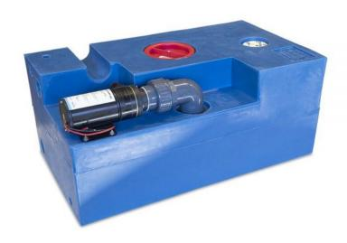
Complete waste water tank kit ready to install. Including a 72L (19 G) rectangular tank in reinforced polyethylene, waste water macerator pump 12V, gas vent, active carbon filter, control panel and probe for level control. Linear low density polyethylene is the best suited material for holding tanks because of resistance to corrosion and odor permeation.
