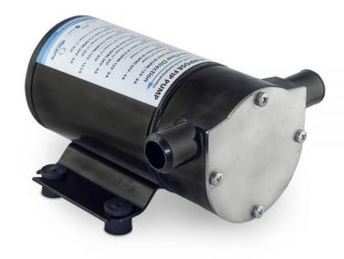
DC 12V F2 size FIP pump with capacity 30 L/min (8 GMP). Used for pumping water, oils and chemicals. Pump body in thermo polymer, stainless steel shaft and PN 06-01-009 Nitrile impeller. Port connections 19mm (1/2"), self priming up to 3m vertical lift. Reversible flow direction, 8A fuse. Interchangeable with Johnson Pump 10-24886-01.
