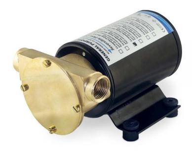
DC 12V F3 size FIP pump with capacity 35 L/min (9,3 GMP). Used for pumping water, oils and chemicals. Pump body in brass, stainless steel shaft and PN 06-01-009 Nitrile impeller. Port connections 19mm (1/2"), self priming up to 3m vertical lift. Reversible flow direction, 8A fuse. Interchangeable with Johnson Pump 10-24516-01.
