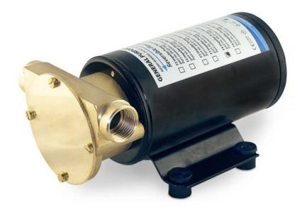
DC 12V F4 size FIP pump with capacity 45 L/min (12 GMP). Used for pumping water, oils and chemicals. Pump body in brass, stainless steel shaft and PN 06-01-009 Nitrile impeller. Port connections 19mm (1/2"), self priming up to 5m vertical lift. Reversible flow direction, 12,5A fuse. Interchangeable with Johnson Pump 10-24689-01.
