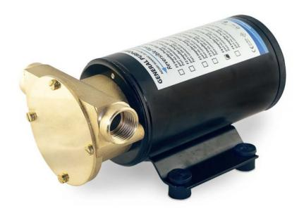
DC 24V F4 size FIP pump with capacity 45 L/min (12 GMP). Used for pumping water, oils and chemicals. Pump body in brass, stainless steel shaft and PN 06-01-009 Nitrile impeller. Port connections 19mm (1/2"), self priming up to 5m vertical lift. Reversible flow direction, 6A fuse. Interchangeable with Johnson Pump 10-24689-02.
