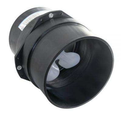
7" in-line mounted marine ventilation 12V axial blower with capacity 1000 m3 per h, 589 CFM. 178mm port connection and 250mm length. Sheltered blades from blower housing interference at tough installation. Compact 5 blade design to maximize performance. For continous duty. 7A fuse. Interchangeable with Vetus Vent17812A.
