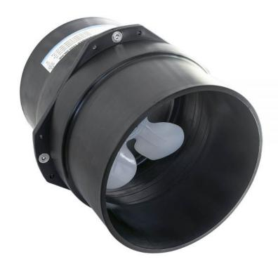
7" in-line mounted marine ventilation 24V axial blower with capacity 1000 m3 per h, 589 CFM. 178mm port connection and 250mm length. Sheltered blades from blower housing interference at tough installation. Compact 5 blade design to maximize performance. For continous duty. 3,5A fuse. Interchangeable with Vetus Vent17824A.
