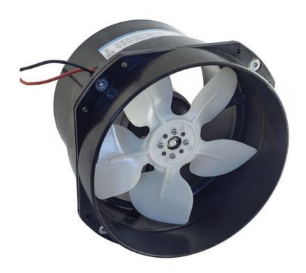
7" in-line mounted marine ventilation 12V axial blower with capacity 1000 m3 per h, 589 CFM. 178mm port connection and 165mm length. Sheltered blades from blower housing interference at tough installation. Compact 5 blade design to maximize performance. For continous duty. 7A fuse.
