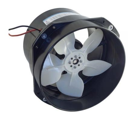
7" in-line mounted marine ventilation 24V axial blower with capacity 1000 m3 per h, 589 CFM. 178mm port connection and 165mm length. Sheltered blades from blower housing interference at tough installation. Compact 5 blade design to maximize performance. For continous duty. 3,5A fuse.
