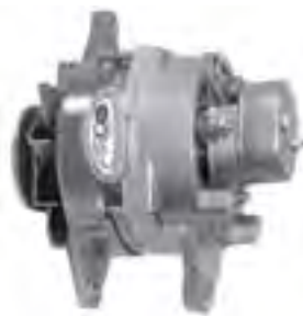
Brush Cover Installed
