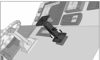
3 Attach your electronic fishfinder or other marine radio to the mounting plate through the AMPS base plate. Choose the screws (not included) that will work best to mount your device.
