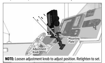
2 Using a screwdriver and/or drill, attach the mounting plate to the pedestal using 4 bolts (not included).
