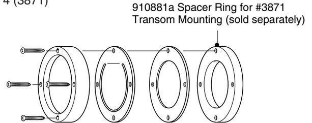
2. Mark holes and drill to accommodate #6 x 1" (25mm) self-tapping screws.
