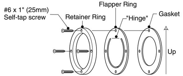
Note: when using the 3871 Scupper Valve for transom mounting, you **must** use a second retainer ring, #910881a, to back-up the flipper valve (figure 4). This part can be purchased separately.
