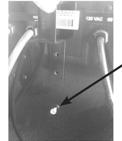
3. Align the cable bracket mounting holes with the upper two handle mounting holes as shown. Install the two screws and fully tighten all three handle mounting screws.
