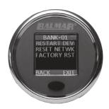
The advanced menu for any SmartShunt allows the user to perform several levels of reset of SmartLInk devices on the network. An explanation of each of options is in the table below:
