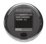
Each SmartShunt on a SmartLink Network has it's own menu. If you only have one SmartShunt, it is automatically selected for you. Otherwise, select the SmartShunt that you wish to configure (Using the long-press method) and then select MENU, and then CONFIG. A complete description of the configuration options can be found in the CONFIG section later in this manual.
