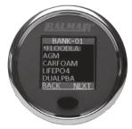
The currently selected battery type is noted with an asterisk (\*) in front of the name. The default is AGM-STD (see the chemistry table). If this is your chemistry and the installation is new, you may either re-select the chemistry, ensuring that the SG200 is starting fresh, or exit back to MENU and move to the next step.
