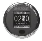
Once you select a chemistry, you must specify the capacity of the battery bank. This is the total design capacity of the entire bank, regardless of the battery's condition, or previously measured capacity. Typically the capacity is expressed as the 20-hour discharge rate. This may be written as something like "105Ah/20h" on the battery or battery documentation. If you cannot find an Ah specification for your battery, but it does show a reserve capacity (RC)
