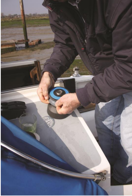
Step 3: Fitting Wincher lip to drum top lip
