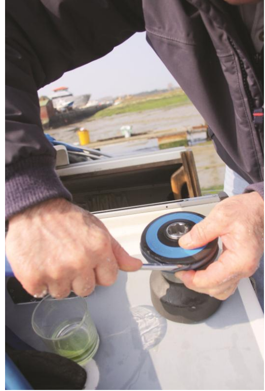
Step 3: Fitting Wincher lip to drum top lip
