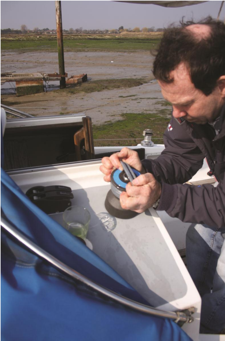
Step 2: Fitting Wincher onto drum
