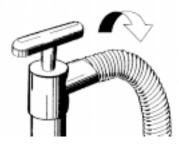
Rotate your right hand back toward you to turn the hose into the thread. Turn the hose into the sleeve until it stops. Give the hose a strong pull with your right hand to make sure that the hose is properly seated into the threaded sleeve.
