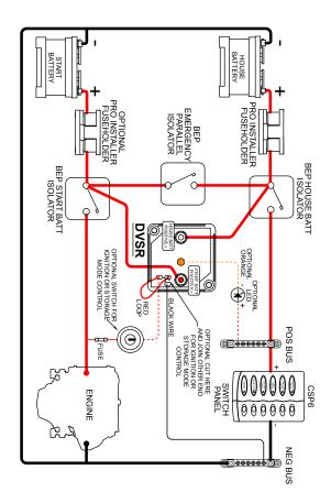
**Example System:** NOTE – This diagram is a guide only showing DVSR connections and not intended as a full electrical systems wiring diagram.
