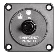
Emergency parallel control is achieved by using a remotely mounted momentary switch, such as the BEP #80-724-0007-00 unit (pictured at left), which also features an LED to show the battery switch status. When operated, the remote switch engages the 720-MDO-EP contacts, paralleling the batteries for a 10 minute period, for example to get an engine started following a flat start battery. Alternatively, the battery switch can be manually over-ridden to either "Manual On", or "Manual Off" modes.
