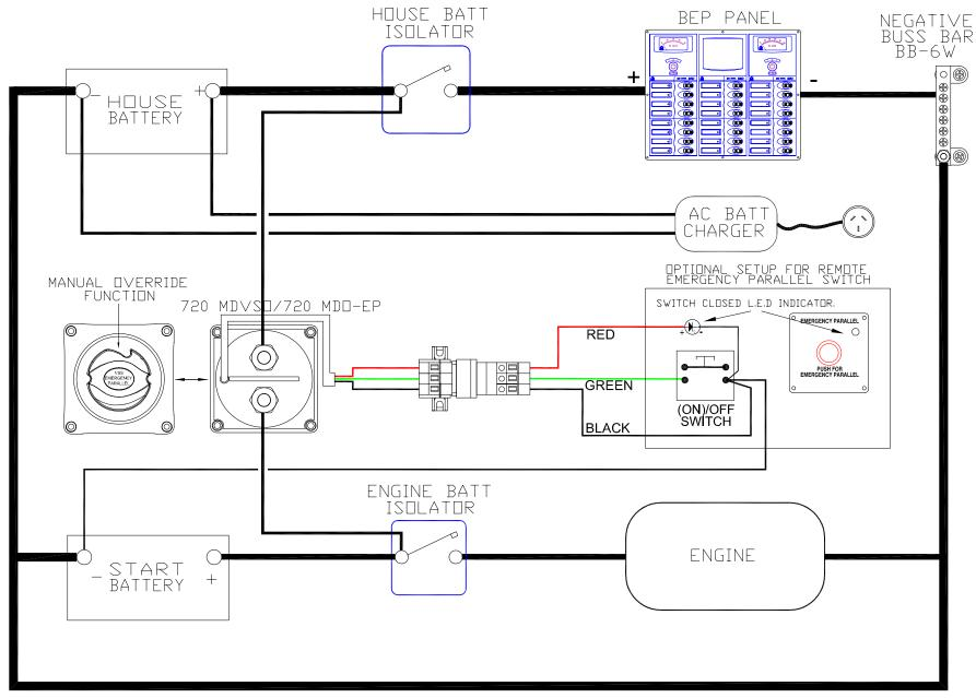
IT IS IMPERATIVE THAT THE NEGATIVE (BLACK) FOR THE MDO-EP/MDVSO IS TAKEN FROM THE SAME BATTERY THAT IT IS ISOLÁTING. FAILURE TO DO THIS WILL CAUSE THE UNIT TO WORK ERRATICALLY. ONLY ONE NEGATIVE MUST BE SUPPLIED TO EACH UNIT FOR CORRECT OPERATION.
