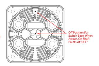
Replacement of Actuator (always remove, and replace the Actuator with knob in the "OFF" position)
