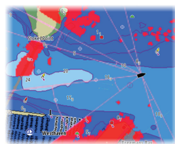
Radar overlay on a chart
