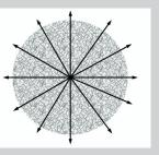
Bird Spider 360° arm "tips" should overhang mounting surface by at least 2".
