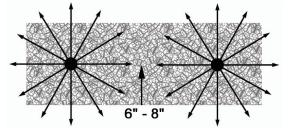
sure that they are installed 6-8" from arm tip-to-arm tip (not base-to-base).
