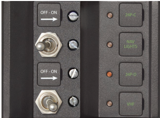
COTS Circuit Breaker (p. 80)
