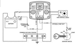
Note: Because the ATD is single sensing the battery must be attached to the stud labeled BATT and the devices to be disconnected must be attached to the stud labeled LOAD. Reversal of these connections will render charge sense functionality non-operational.
