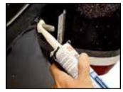
**2.** Prep your transom for the jack plate installation. Remove any old silicon or chalk. Apply marine sealant around each bolt hole and a bead around the jack plates mounting flanges.
