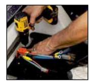
**4.** Mount the relay box in as dry a location as possible but within 4' of the battery using stainless steel hardware or wire ties (not provided).
