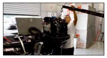
**1.** Using a safe and proper lifting method carefully remove your outboard motors mounting hardware from the transom and swing the outboard away from the transom.
