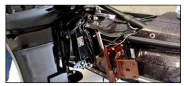
**11.** Mount your outboard motor to the jack plate. (It may be necessary to raise the jack plate all the way up to allow for clearance to install the lower mounting bolts.) Use the engine manufactures' recommended mounting torque and repeat step 10.
