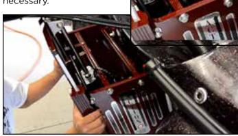
NOTE: It may be necessary to install the wiring harness before bolting the motor to the jack plate. Move the jack plate up for clearance to install the motor to the jack plate.
