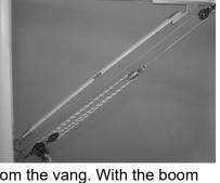
as a guide. Use Locktite on threads. **Hint:** Once installed, to attach the Boomkicker, it's usually easier to slide the Boomkicker into the boom track first, then attach it to the mast fitting, rather then attaching to the mast first.
