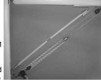
**2.** <u>Position Boomkicker:</u> The Boomkicker works by flexing upward and when straight, it is at the top of its travel. Install the Boomkicker with the
