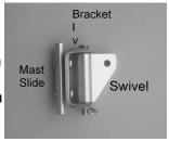
**5.** <u>Install Boom Fitting:</u> Make sure the rod clamps at both ends are tight. Then attach the Boomkicker to the mast fitting, and the slide and track at the boom end. The angle on the track goes forward, the stop in aft. <u>Important:</u> The vertical edge of the slider must be forward to allow flex room for the Boomkicker. There are 3 standard choices for the stop with the initial position in the middle
