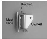
**5.** <u>Install Boom Fitting:</u> Make sure the rod clamps at both ends are tight. Then attach the Boomkicker to the mast fitting, and the slide and track at the boom end. The angle on the track goes forward, the stop in aft. There are 3 standard choices for the stop with the initial position in the middle for later adjustment if needed. If necessary
