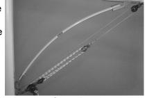
through the groove. Use the 1/4" drill and the 5/16-18 tap provided, with the mast fitting bracket as a guide. A variable speed, reversible drill makes tapping easy. Go slow. Locktite is recommended on threads.
