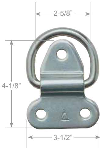
1/2" Hinged Pad Eye Safe Working Load: 3500 lbs
