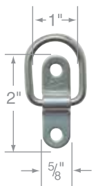
3/16" Hinged Pad Eye Safe Working Load: 400 lbs
