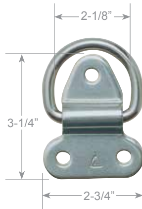
3/8" Hinged Pad Eye Safe Working Load: 2500 lbs
