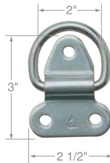
5/16" Hinged Pad Eye Safe Working Load: 1500 lbs
