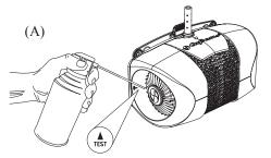
**2. Freezer Test:** Ensure the Pali is unplugged and cooled down. Place the heater in a plastic bag and into a freezer. This will lower the temperature of the thermostat. After 2 hours, remove the Pali from the freezer, remove plastic bag and plug in. The heater will automatically activate indicated by the LED turning red.
