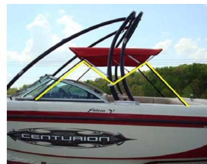
Placement of the hold-down straps should form the letter "M". Straps should form a 45 to 90 degree angle with each bow.
