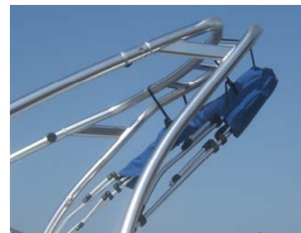
Tower Bimini, Stored Position
