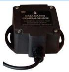
The sensor which is gimballed for plus/minus 45 degrees of pitch and roll, is mounted in a position where stray magnetic fields are at a minimum. An electronic auto calibration then cancels out small errors.
