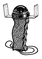
**Sighting Objects.** Hold the compass in a relaxed position at arms length, with the yellow cursor line facing you. With the compass slightly tipped so both pointers are visible, rotate your arm and upper body until both pointers are in-line with the object being sighted (figure 1). Read the magnetic bearing as it appears at the yellow cursor line.
