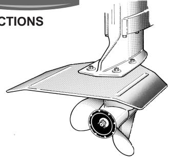
Whale Tail XL mounts on the anti-cavitation plate of all inboard/outboards and outboards. Installs in 15 minutes with stainless steel hardware included. Made of marine grade aluminum with durable anodized finish.
