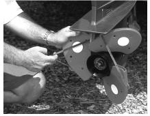
**2.** Secure blade covers with the rubber cinch strap stretched onto all three locking tabs. This holds the blade covers securely together for trailering.
