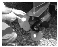
**1.** Put rubber cinch strap over the hub of the propeller and slip blade covers onto propeller blades with each reflective dot facing out.
