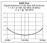
In conjunction with the USCG Automatic Identification System (AIS) requirements for commercial vessels, Digital Antenna created a series of 4' AIS antennas that meet the exacting AIS frequency requirements. Designed with a low 1.5:1.0 SWR ratio from 159-162 MHz, Digital Antenna's 4.5 dB gain AIS antennas offer unsurpassed durability and performance compatible with all AIS transponders.
